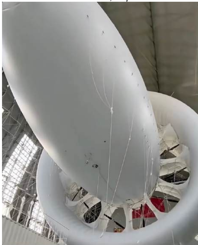
S1500 view from under the main hull looking aft toward the inflated annular duct structure. Source: Screenshot from YouTube video, Sep 2025
