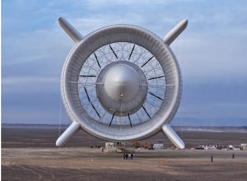
Stern view of the S1500 moored outdoors, showing all twelve 2-bladed air turbines positioned inside the annular duct. Source: South China Morning Post
