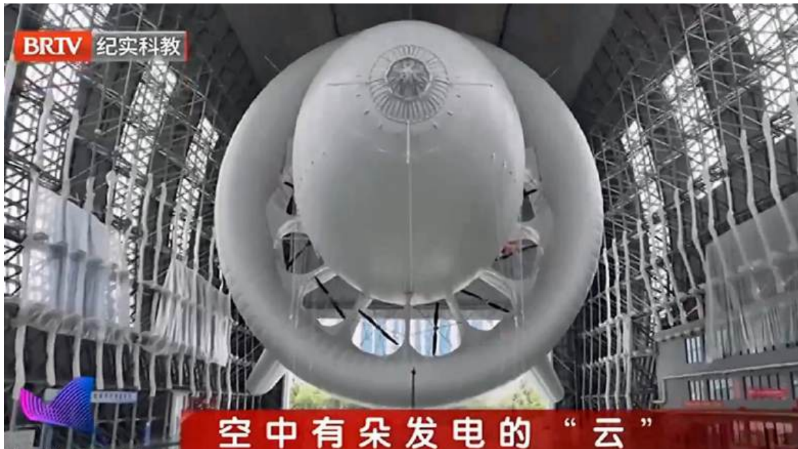
S1500 bow-on view showing the geometry of the central hull and the inflated annular ring structure housing twelve 100 kW micro-turbines, each driven by a two-bladed carbon fiber turbine. Source: BRTV (China) via screenshot from YouTube video, Sep 2025
