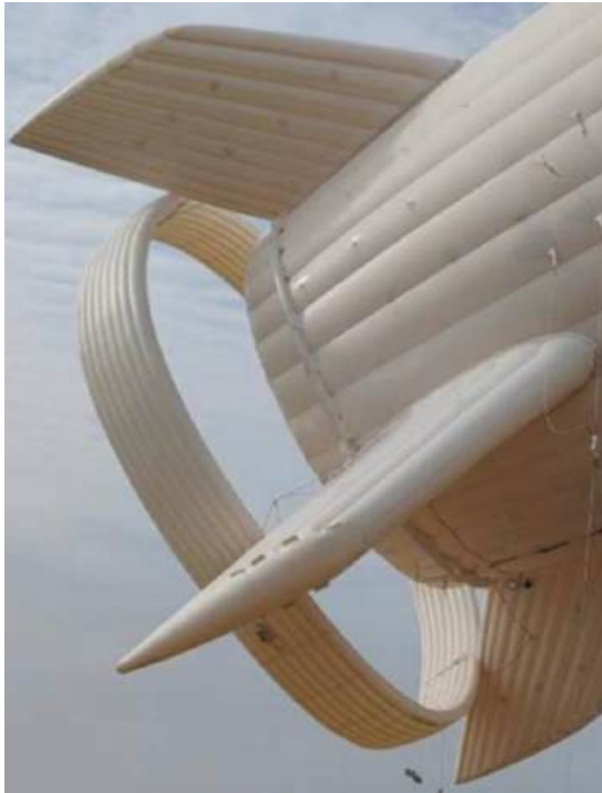
Details of the S500 ring tail configuration. Source: (L) China Daily (10 Oct 2024), (R) Screenshot from New China TV video (17 November 2024)
