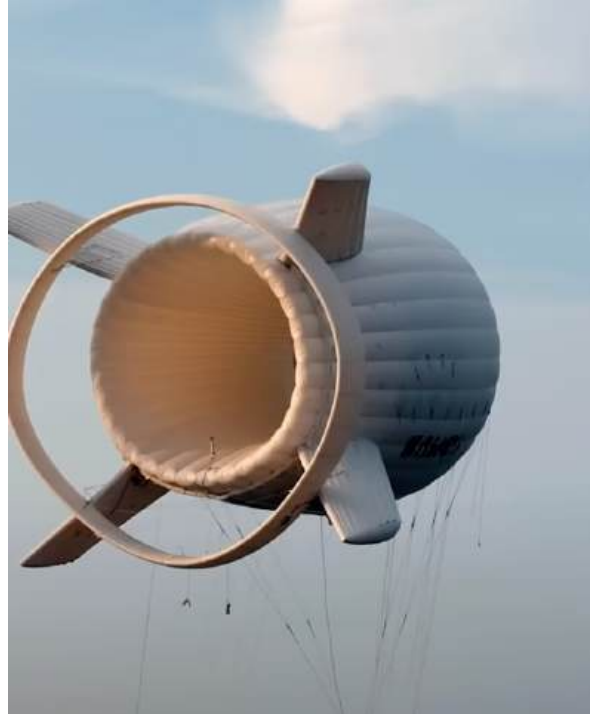
Details of the S500 ring tail configuration. Source: (L) China Daily (10 Oct 2024), (R) Screenshot from New China TV video (17 November 2024)
