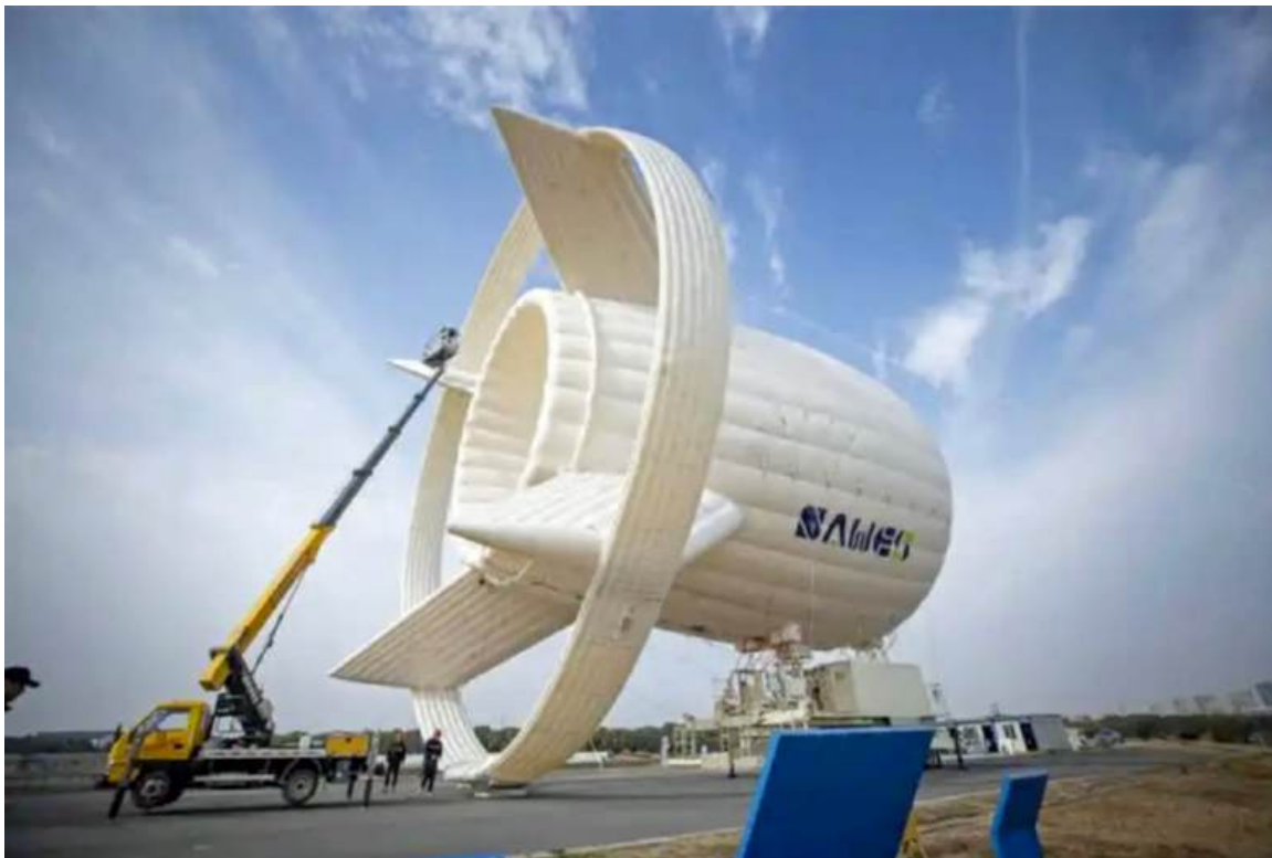
S1000 on the ground, docked on its base station. Note the revised ring tail configuration. Source: Screenshot from YouTube video
