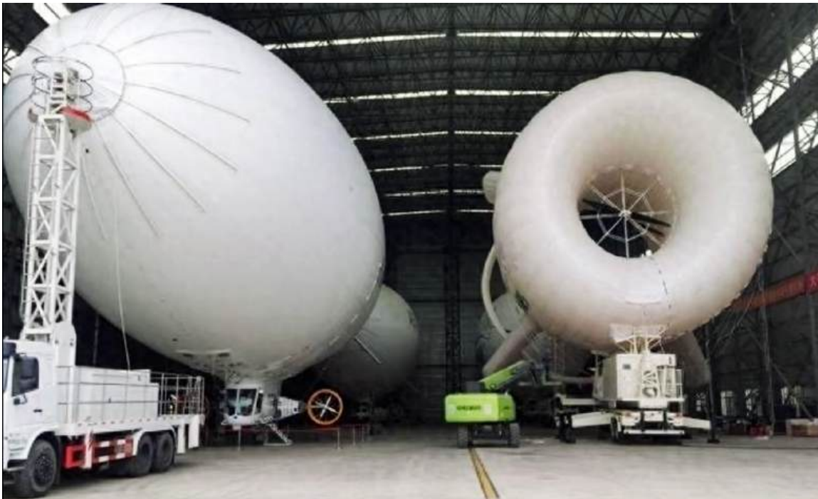
S500 SAWES and its base station (right) in a hangar with an AVIC AS700 blimp. Source: Screenshot from New China TV video (17 November 2024)
