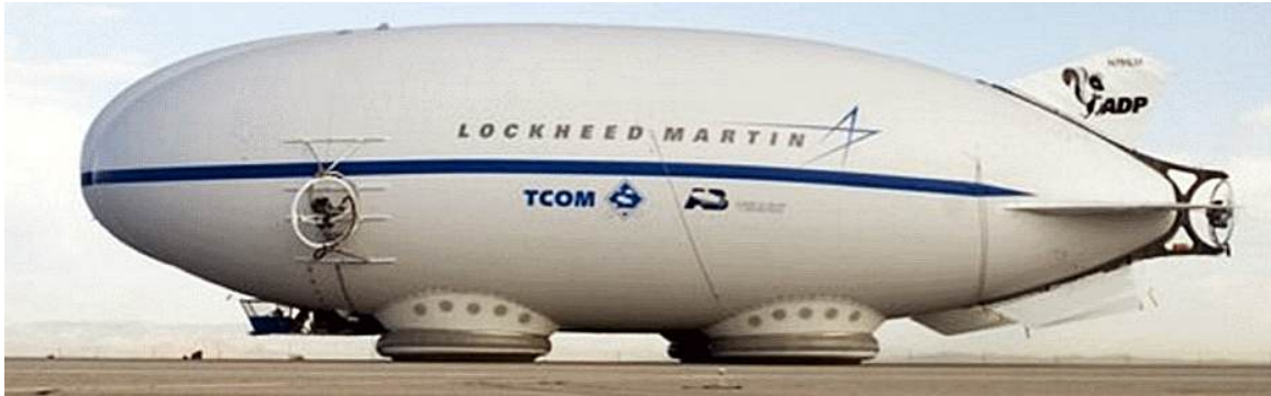
Profile view of the P-791 on the ground. Source: Lockheed Martin
