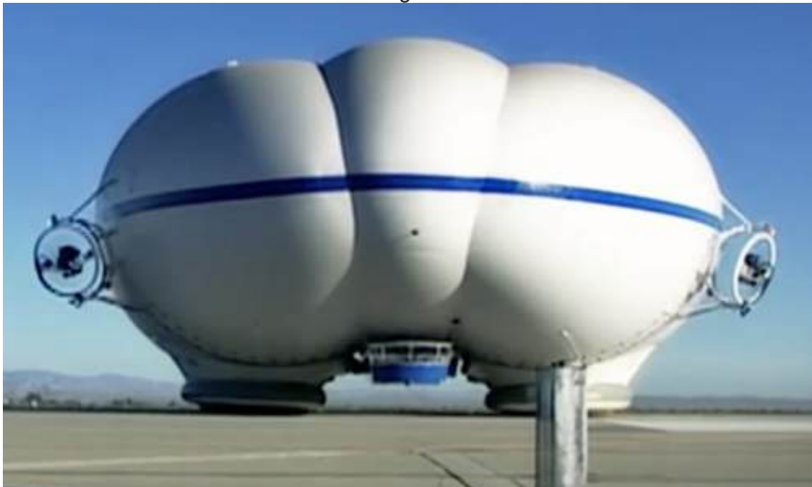
Bow view on the ground, showing the tri-lobe hull design, the gondola under the envelope's centerline, and the two flank-mounted thrust vectoring propellers. Source: Screenshot from Lockheed Martin video.
