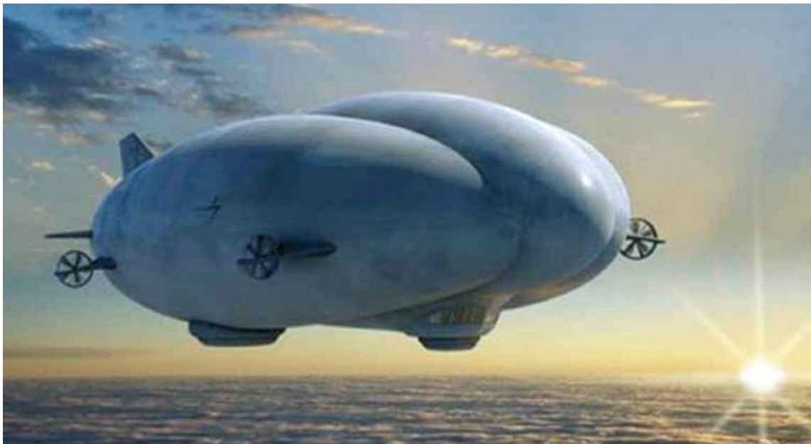
Lockheed Martin LEMV design concept, with significant changes for the P-791 & PERSIUS configurations (i.e., aft flank-mounted propellers, three-pad ACLS) Source: Lockheed Martin via NAA Noon Balloon (Winter 2009)
