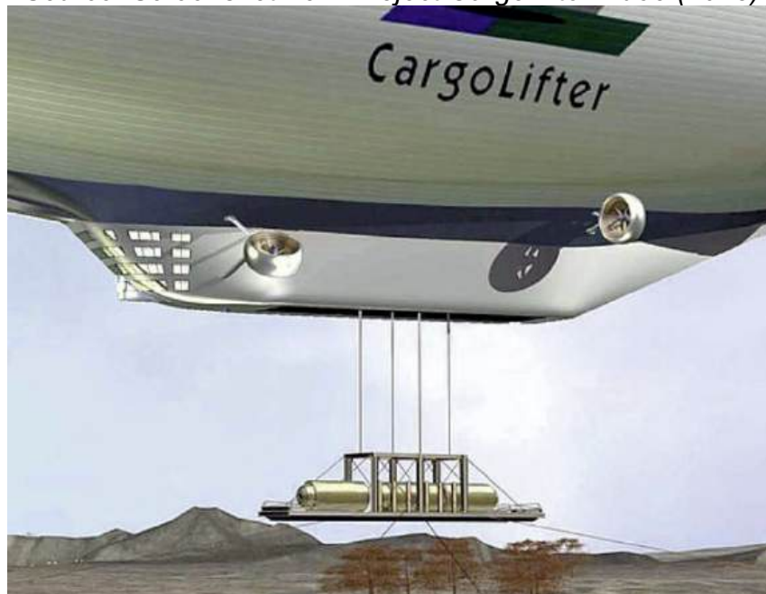
Load frame supported by four hoist cables and stabilized with four tethers. Source: CargoLifter AG
