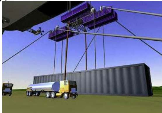
(L) Water tanker truck approaches & starts delivering water ballast to the load frame. (R) Water trucks have delivered sufficient ballast water to transfer the load of the cargo to the ground. About 42,250 gallons of water (7 to 9 semi-trailer tanker trucks) would be needed for a 160 metric ton load transfer.
