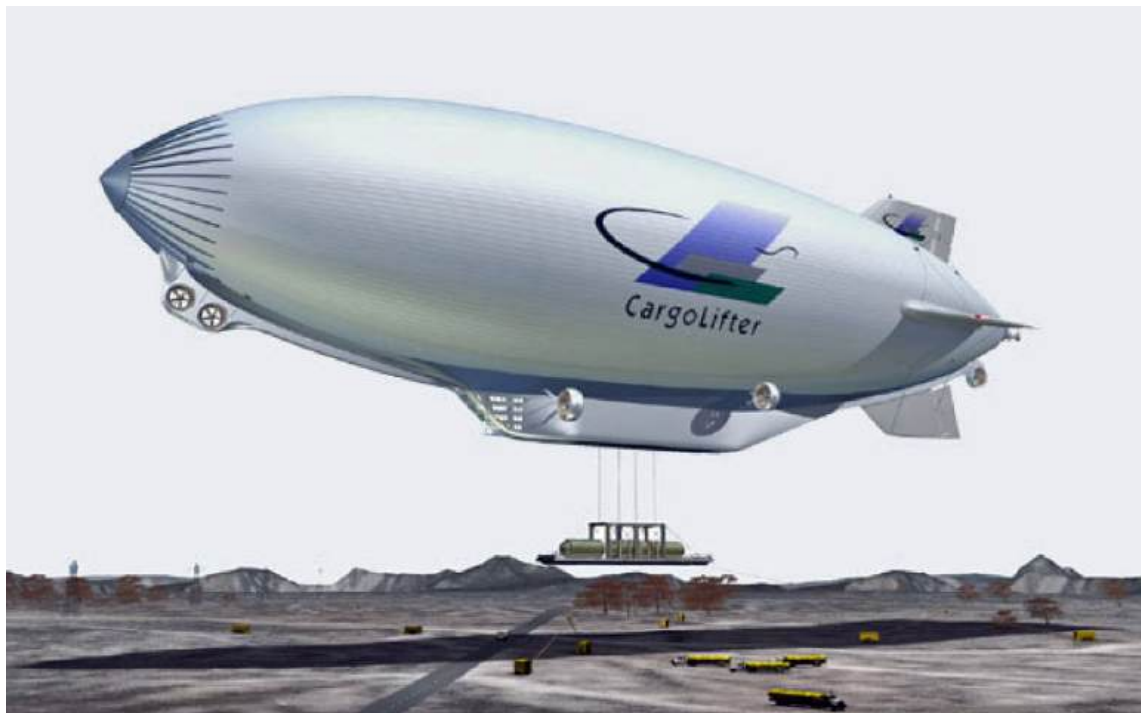
Load exchange in progress from a CL160 (final generation) hovering at about 100m (328 ft). Source, both graphics: CargoLifter AG
