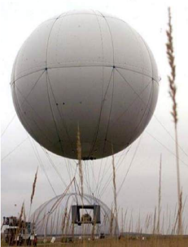
CL75 AC aloft on tethers during May 2002 load test with the mine-clearing tank. Source: CargoLifter AG Pics from cargolifter.com
