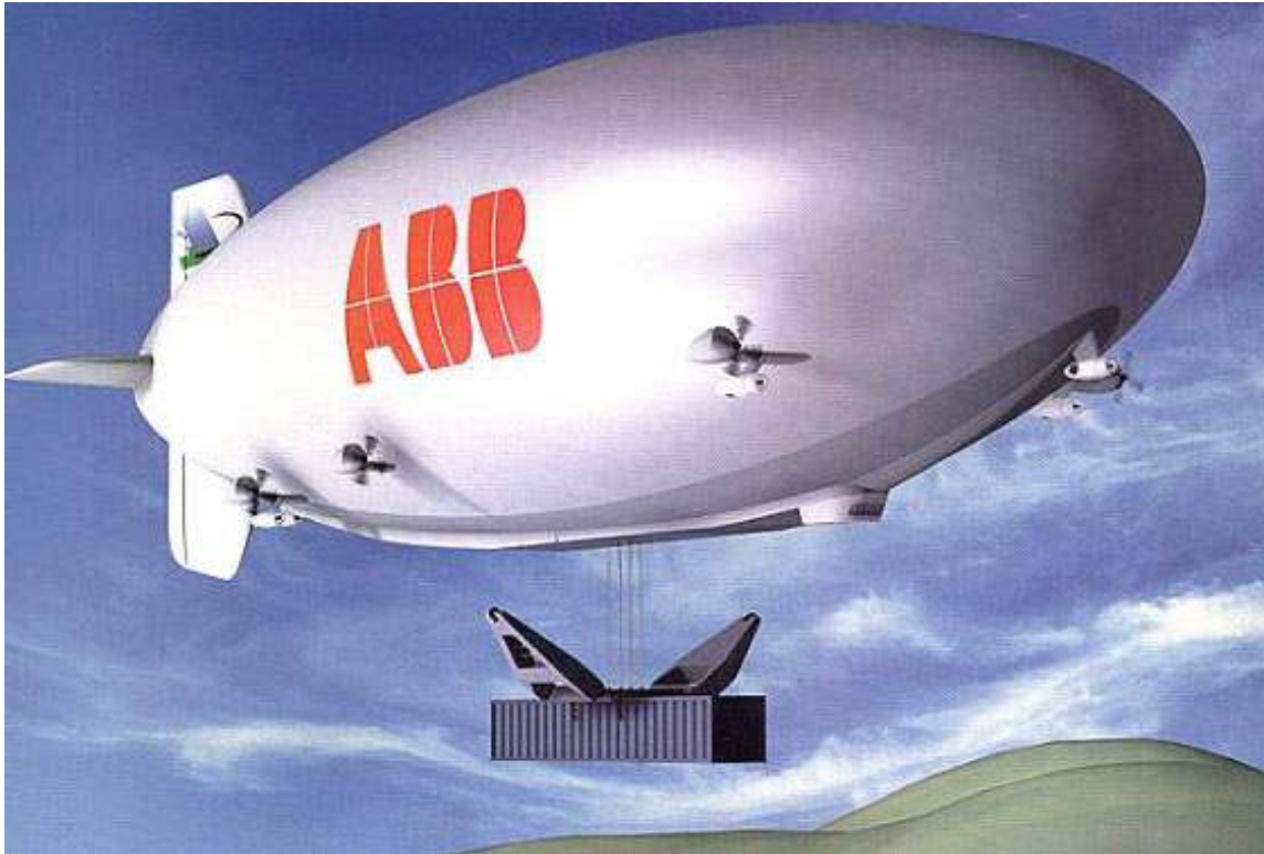
Early generation CargoLifter variant, with an alternate main propulsion and maneuvering thruster arrangement, carrying a large cargo item as an external sling load. Source: CargoLifter AG via Aerospace Technology (July 2002)
