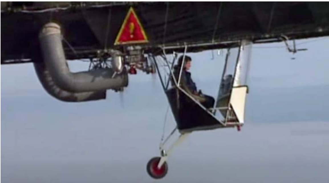
Joey two-seat cockpit & twin engine installation, with envelope air supply ducts in the propeller slipstreams. Source: Screenshot, Joey-Testflug video (2008)
