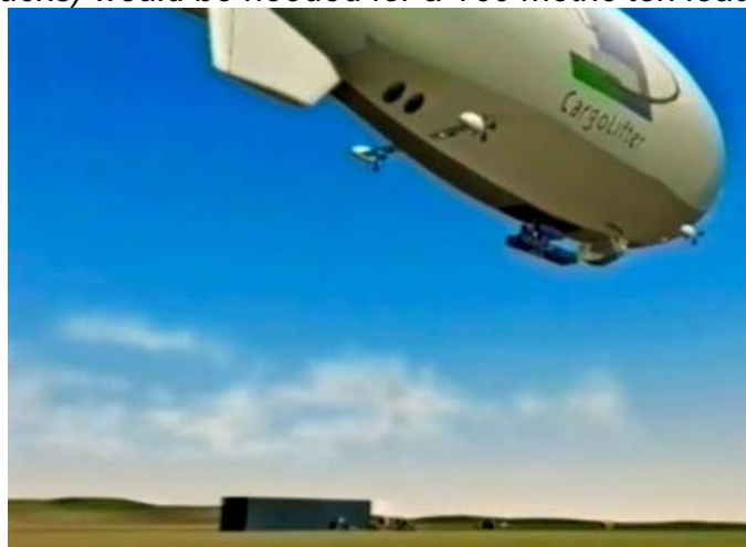
Cargo on the ground, load frame disconnected and being retracting as airship leaves the site after delivery. Source, four graphics: Cargolifter AG, via screenshots from promo video (2001).
