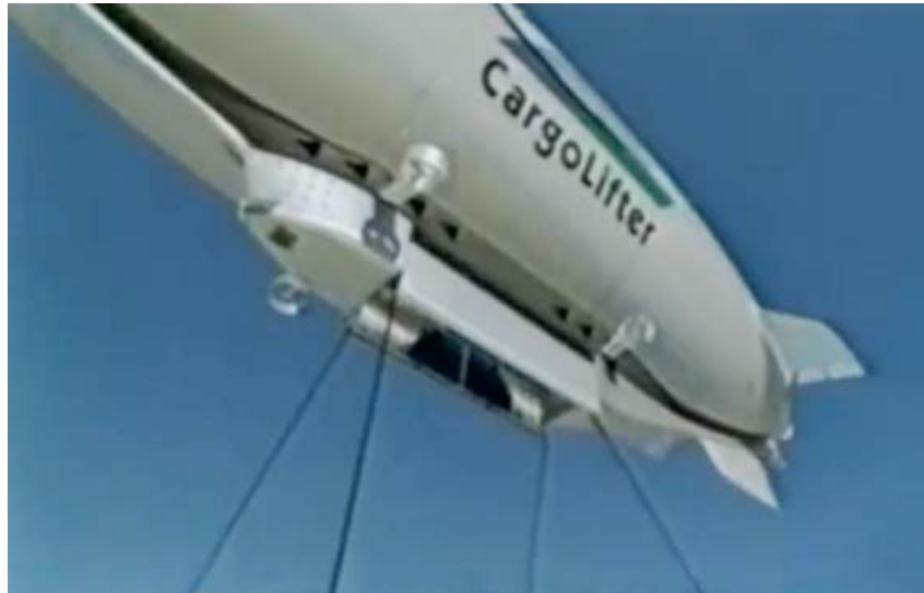
Starting to lower the load frame with four tethers deployed. Source: Screenshot from Project CargoLifter video (2013)
