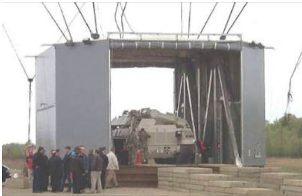
German mine-clearing tank inside the CL75 AC load frame. Source: cargolifter.com
