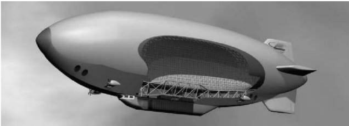
Early generation CL160 cutaway drawing showing the keel structure extending along the bottom of the envelope. The cargo bay is the dark area in the center of the long gondola. Source: Carl Schweizerhof / Wilhelm Rust, "Finite element load limit analysis of thin-walled structures....." July 2002
